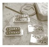
And the internal parts are just horrible. They have these really thin nylon bobbins that are extremely heat sensitive. They heat-pressed in a little metal stud that they attached the coil wire to, and it melts very easily and will break the coil. There are just so many things
