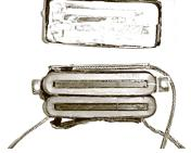
Firebirds have a bar magnet in each coil. The absence of steel inside the coil changes the inductance, which in turn affects output and frequency response. The overall tone of the Firebird is more like a single coil – less bass, brighter
